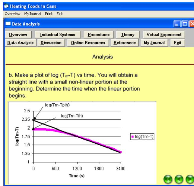
Figure 1.7. Data analysis for determining heat transfer parameters in foods during canning.
