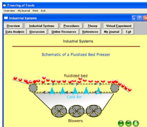
Figure 1.6. An animated view of an industrial fluidized bed freezing system.
