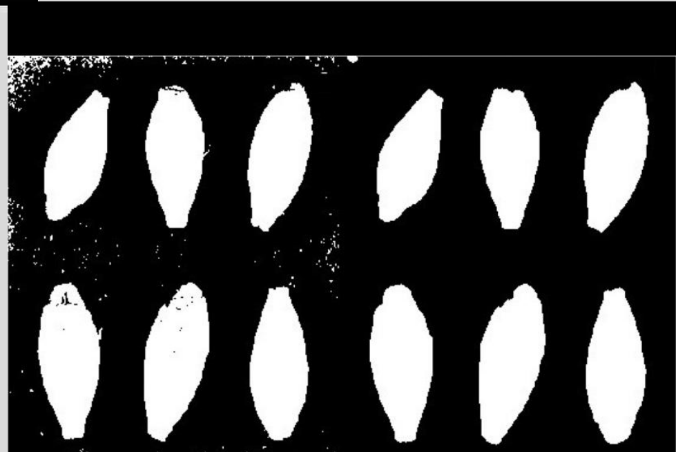
The result of the segmentation (a) after the image gray-scale thresholding and (b) followed by morphological closing and opening
