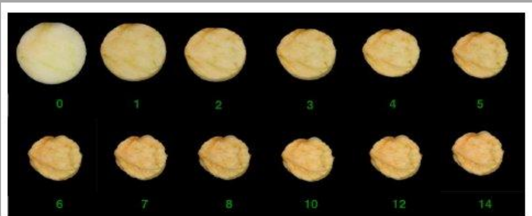
Fig. 2. Gallery of images of a single apple slice as a function of drying time (time in hours).
